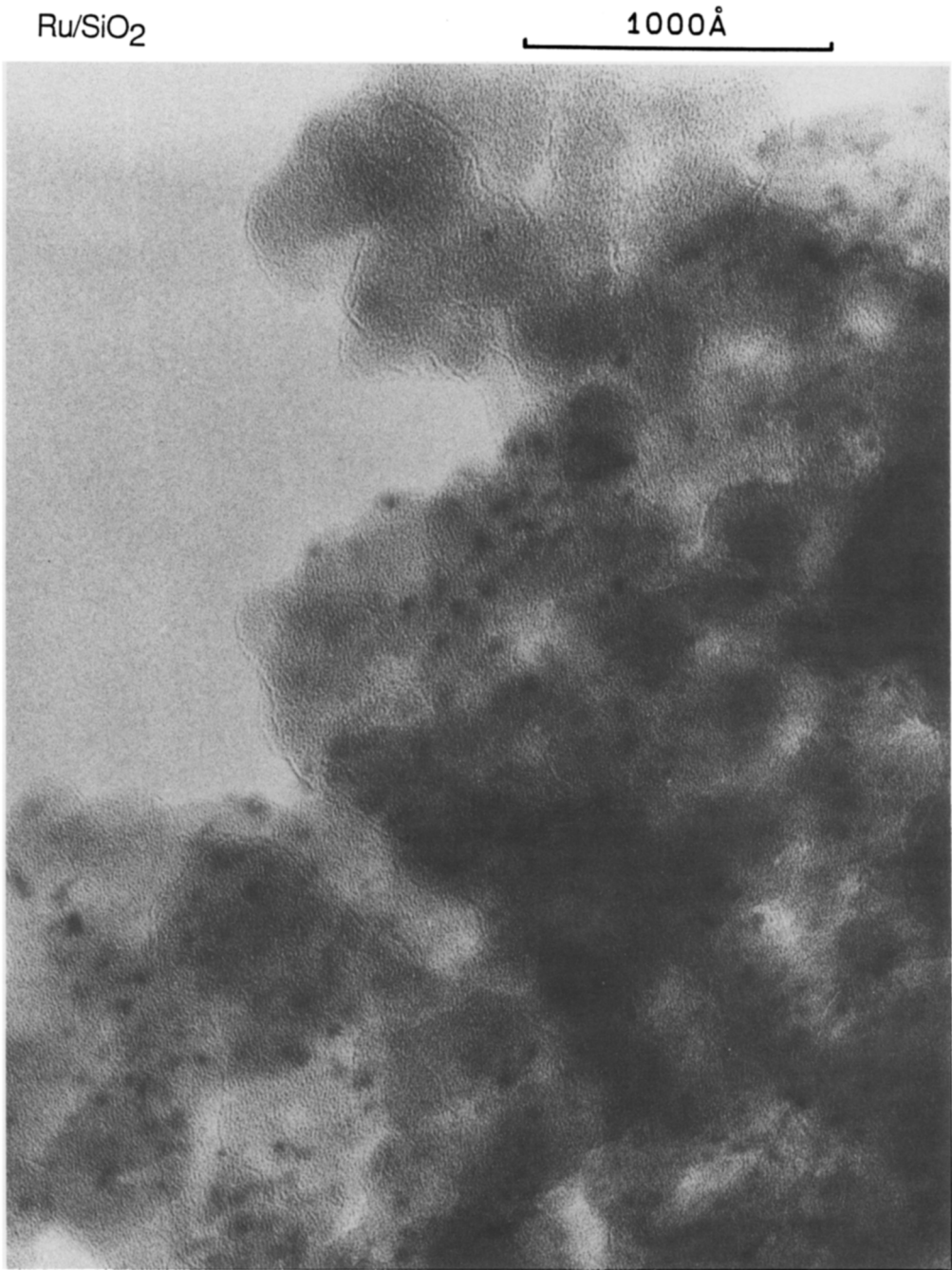
FIG. 2. Electron micrographs of \text{Ru}/\text{SiO}_2 , \text{Ru}/\text{TiO}_2 and \text{TiO}_2/\text{Ru}/\text{SiO}_2 catalysts (as prepared).
